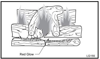
Fig. 69 Correct flame pattern, Models 2950, 2951.
